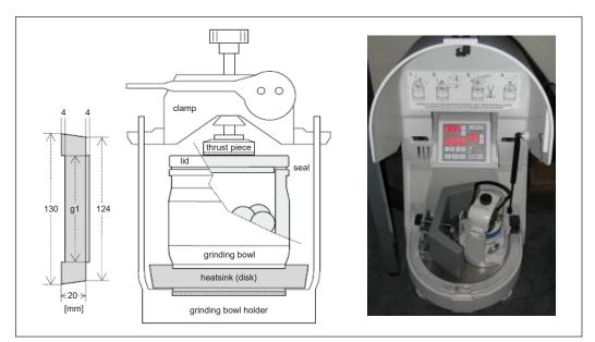
Figure 1. Planetary mill
