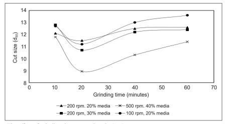
Figure 4. The effect of grinding time to cut size,  $d_{50}$  (µm)
