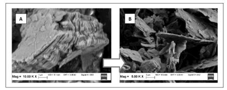
Figure 5. Breakage mechanism applied on mica (A) and delaminated into a layered structure (B)
